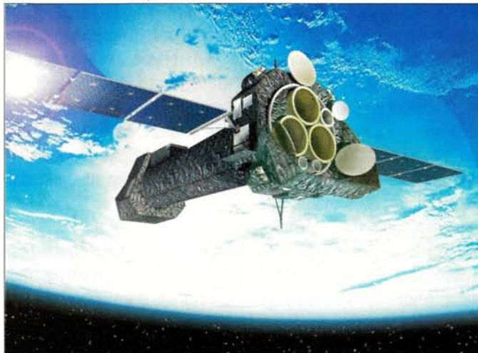
X-ray observatory: artist's view of XMM-Newton in orbit. The openings on the front are the three mirror systems; the detector systems are located at the far end. The satellite is almost 11 m long, with a total solar-panel wingspan of 16 m. (ESA.)
