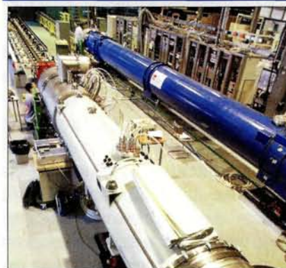
Testbenches for LHC magnets at CERN for 15 m dipoles (background) and a quadrupole (foreground).
