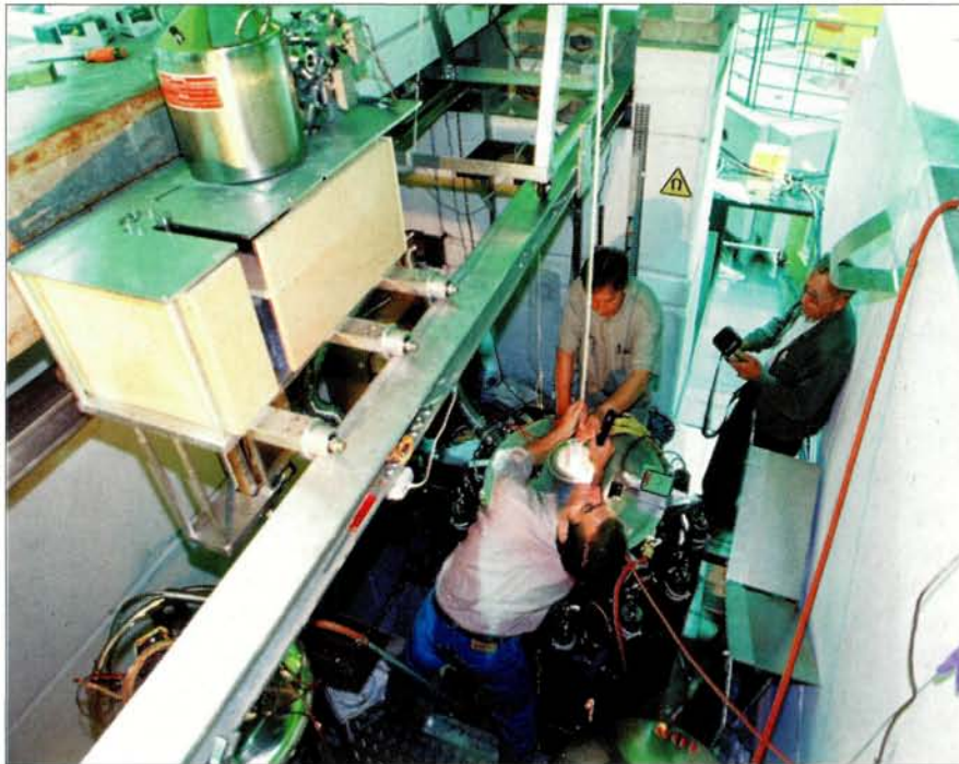
Installing the ATRAP experiment at CERN's antiproton decelerator. Trapping antiprotons using electromagnetic fields provides a cost-effective way of exploiting precious antiprotons.
